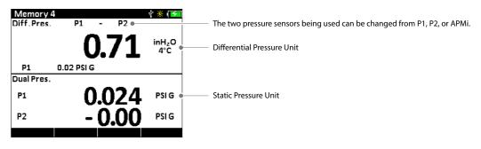
Note: The static pressure is also displayed on the bottom of the window. The unit for the static pressure does not have to be the same as the differential unit.
