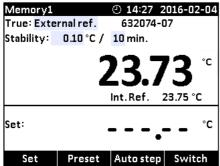
The functions in the horizontal menu bar are available using the Functions soft keys F1 - F4. For Operating principle – See section 5.1.
