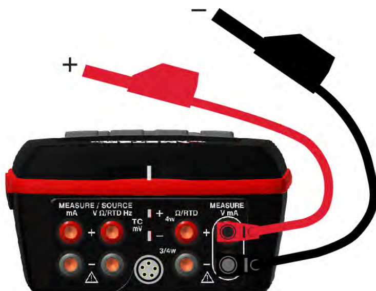
Figure 13 mA current measurement connection (upper window)
