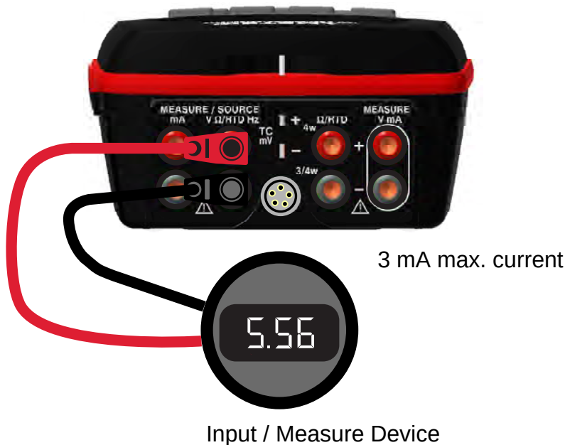
Figure 18 Connections for Testing an Output Device
