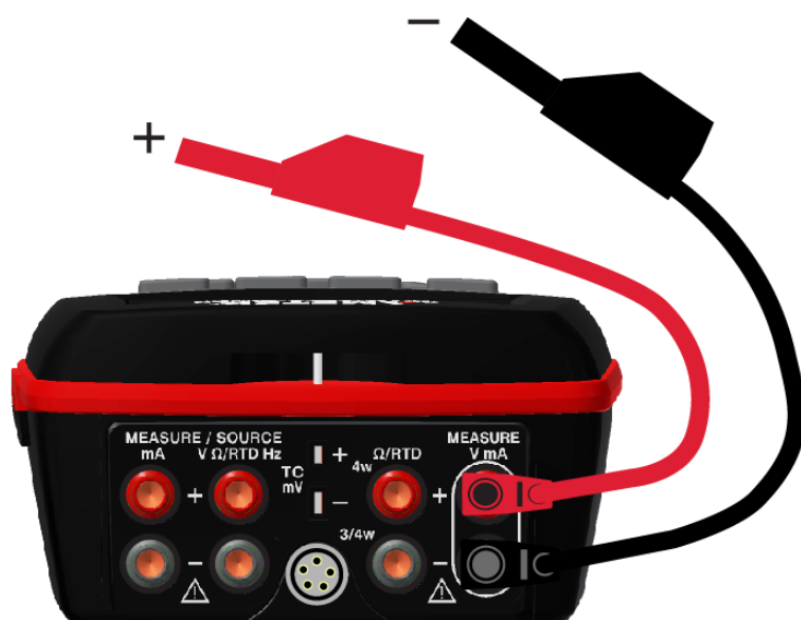
Figure 13 mA current measurement connection (upper window)
