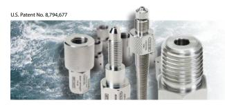
**Fittings for Life** Crystal Pressure Fittings operate up to 10 000 psi / 700 bar with only a finger tight connection needed. Manufactured to be the safest fittings available, CPF are machined in highstrength 316 Stainless Steel, include laser markings to clearly identify fitting type and size, and feature a self-venting weep hole that alerts you before you disconnect from a pressurized system.
