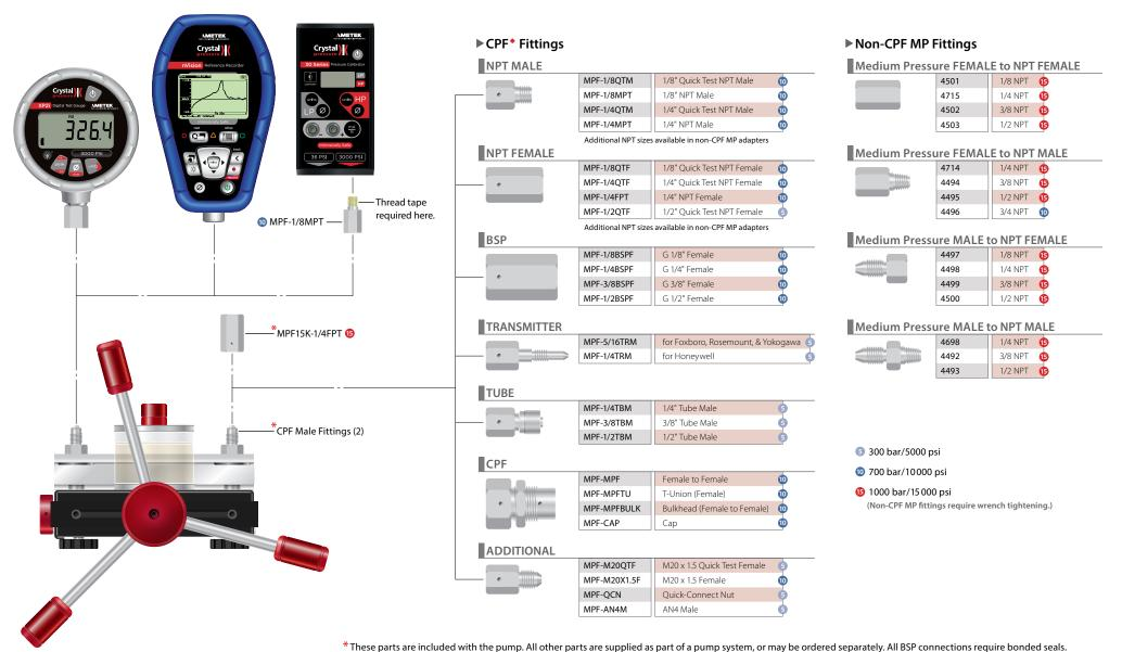
5188.C GaugeCalHP Connection Diagram
