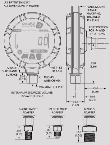
ADDITIONAL SENSOR LENGTH WITH OPTIONAL FITTING ADAPTERS
