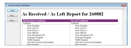
The As Received / As Left Report is a summary of the gauge configuration before and after any changes made using ConfigXP. The As Received state is the condition of the gauge after the initial connect. The As Left state includes all changes since the initial connect, including any changes not yet written to the gauge.
