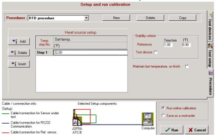
The 3<sup>rd</sup> and final stage of the **calibration setup** is to define the temperature steps called procedures.
