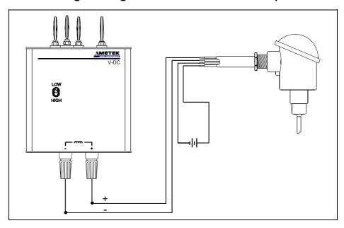
**1.** Connect the 2 transmitter cables to the V-DC module as shown on the diagram.
