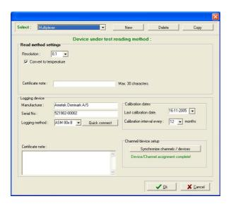
When a user-defined method is selected the logging device section of the dialog is visible to enable the user to define the logging device. Example DTI, DTI050, ASC, ASM-80x or manual.
