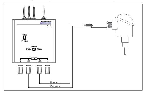
1. Connect the two sensor cables to the RTD module as shown on the diagram.
