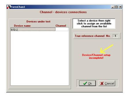
The "Device name" lists contains the test device(s) in the calibration and their assigned channel number.
