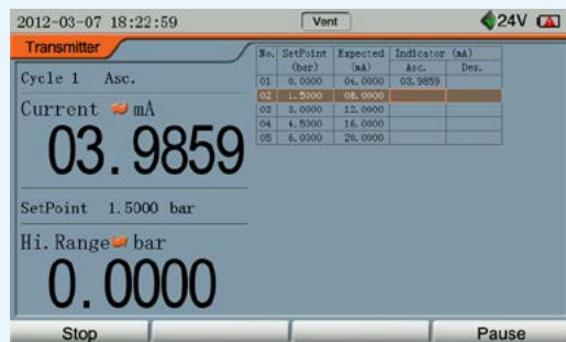
Pressure gauge / transmitter / switch calibration
